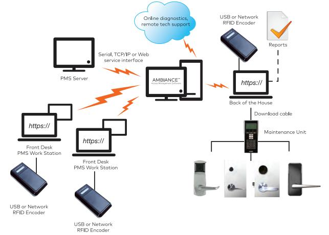
\* Network RFID encoders communicate directly to the server and require an open port on the server to connect.
